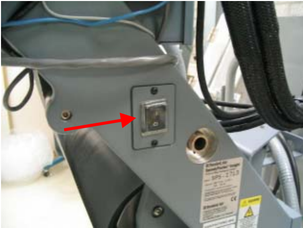
1) Turn OFF the SpeedyPacker and open the front cover.
