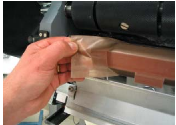
4) Remove the old Teflon tape from the rear sealing jaw.
