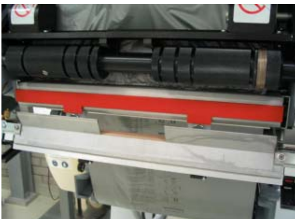
5) Push the orange rubber pad back in the rear sealing jaw.
