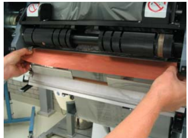
6) Remove the protective plastic from the adhesive area, and place the adhesive part of the tape on the angular shaped part of the rear jaw, located just above the rubber pad.
