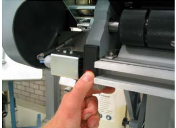
2) Lower the front sealing jaw by unlatching the black/red brackets.
